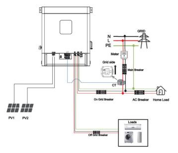
Hybrid inverter are designed for single phase grid.Voltage is
