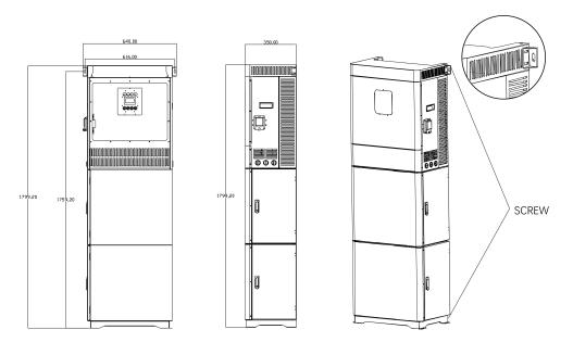
Step 2:The battery fixing, as shown in the figure, push from the right, and a total of 8 M5\*12screws are used. Please pay attention to the direction when assembling the battery.
