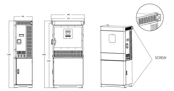
Step 2:The battery fixing, as shown in the figure, push from the right, and a total of 8 M5\*12screws are used. Please pay attention to the direction when assembling the battery.
