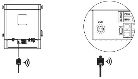
Step1.Plug Wifi into "WiFi" port at the bottom of the inverter.
