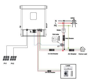
Hybrid inverter are designed for single phase grid.Voltage is 220/230/240V, frequency is 50/60Hz.
